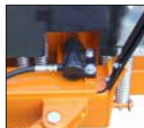
Martinetto "ICE SCRAPER" (OPTIONAL) Device for ice scraping (OPTIONAL)
