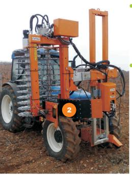
The pre-pruner MP 122 can be optionally equipped with an automatic opening on passage of pickets with detection by infrared scanning or inductive sensors. These two systems each have their specific characteristics.
