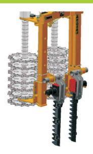
Pair of lateral cuts allows cutting the sides of vines in cordon. They are delivered with a manual setting of the cutting angles and width. Connected in series with the pre-pruning head, they do not require additional oil flow.
