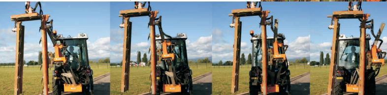
By actuating a single control, the machine can be offset without modification of its seat. The extent of this amplitude allows :
