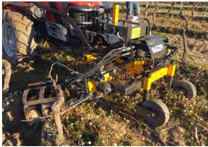
ENERGY DUAL/T con dischiera scolmatrice - ENERGY DUAL/T with plough discs
