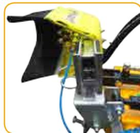
Weeding double bar frontal installed to the tractor via fast creed or on front lift. Provided with two bells of 25 cm, 50 cm or 65 with dual adjustable anti drip nozzles, all with anti-drift bristles for the protection of the product from atmospheric agents or other.
