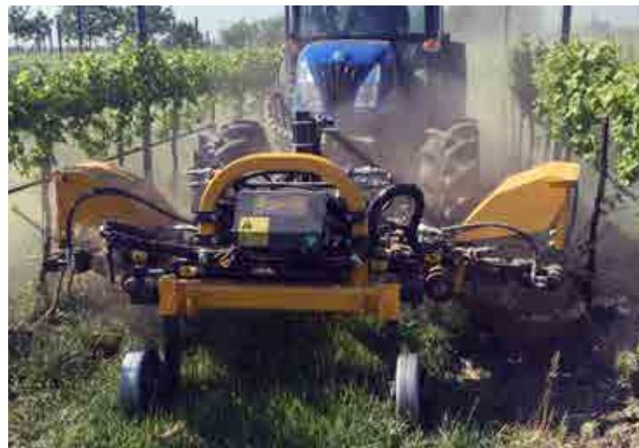
FAST con la testata spollonatrice - *FAST with shoot removing head*
